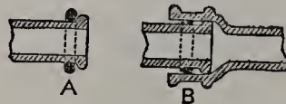
FIG. 99.—Section of india-rubber ring joint. A Ring before, B Ring after, insertion between socket and spigot.
